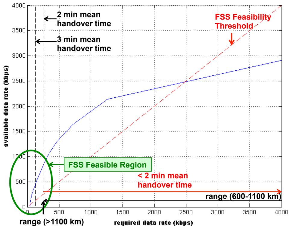
Figure 4 FSS feasible region determination by comparison of available/required data rate
