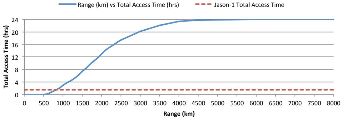
Figure 2 Maximum allowed slant range (km) versus Total access time (hrs)
