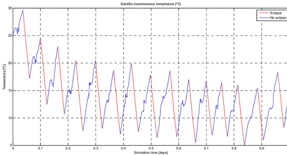
Figure 2: Thermal Budget for a 24 hours simulation in an inclined 55° orbit. The simulation considers 2 ground stations to download data where the S-band and the UHF links are active and three 1000 km radius target areas where both payloads are acquiring data. The figure explicitly shows eclipse phases during the orbit and the consequent drop of the satellite's temperature. The figure is timely connected with the Power budget shown above.
