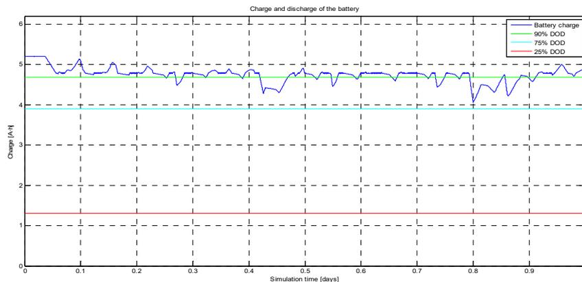
Figure 1: Power Budget for a 24 hours simulation in an inclined 55° orbit. The simulation considers 2 ground stations to download data where the S-band and the UHF links are active and three 1000 km radius target areas where both payloads are acquiring data.
