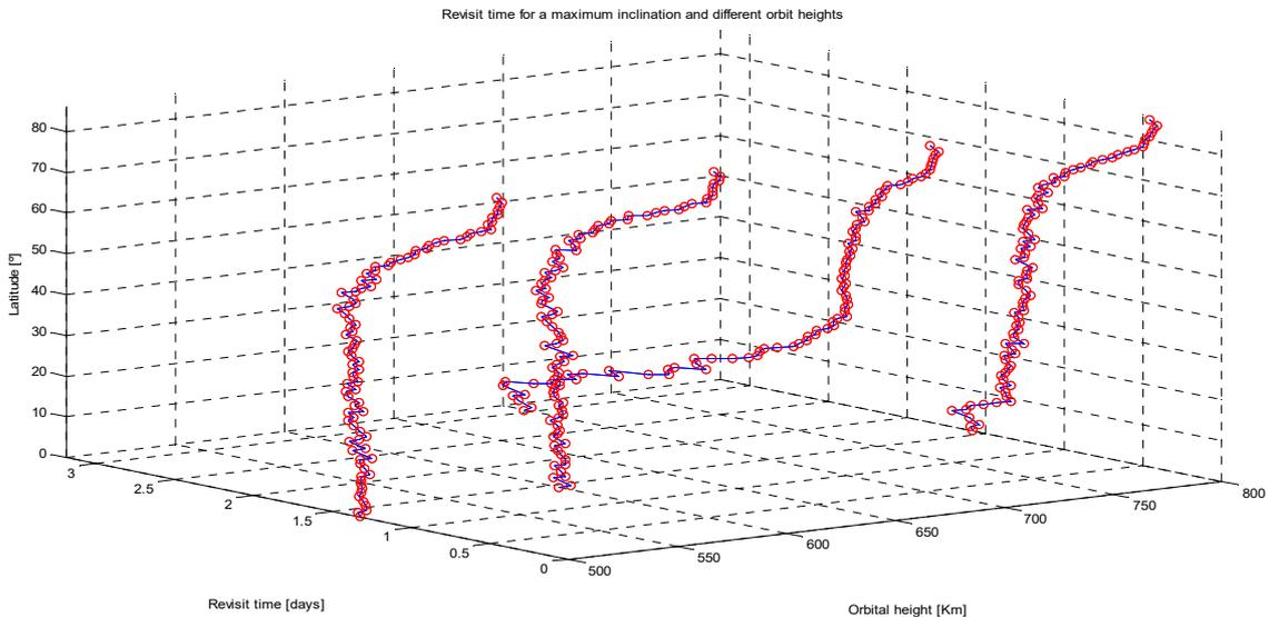
Figure 4: The figure above shows the revisit time for a  $80^\circ$  inclination satellite targeting a random target area with a cross-track swath of 80 Km and an along-track swath of 50 Km. The figure also shows the same experiment for different orbital altitudes and inclinations.
