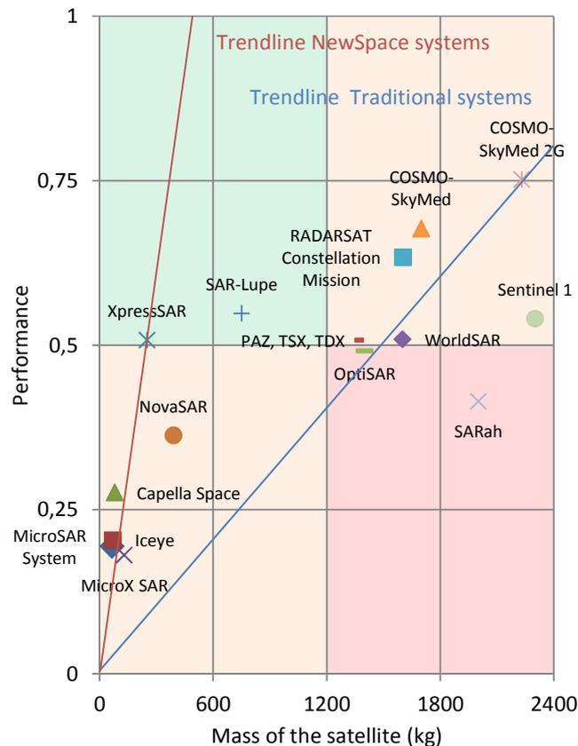
Figure 2: SAR Satellite Performance Index As A Function Of Satellite Mass
